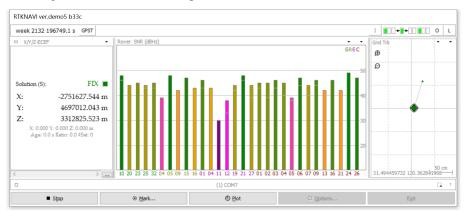
Click the arrow button to switch view (SNR bar, sky map, positioning coordinates, horizontal error scatter, position error timeseries in north, east and up).
