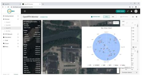
6. **Data Logging and Parsing**: when the device is connected with the PC via the micro-USB cable, the running Python driver is logging all serial port output into files, including raw GNSS/IMU data, positioning solution and the device configuration. These files are located in a subfolder labelled ".pythondriver-windataopenrtk\_log\_xxxxxxx\_xxxxx", e.g.
