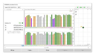
Click the arrow button to switch view (SNR bar, sky map, positioning coordinates, horizontal error scatter, position error timeseries in north, east and up).
