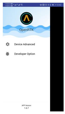
• Click "Device Advanced": user can change and save OpenRTK330 device settings, like Bluetooth ID, lever arm and so on.
