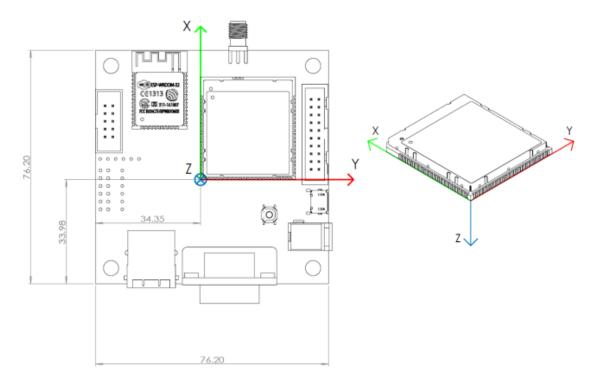
The following mechnical drawing shows the dimension (in mm) of the mounting plate for the OpenRTK330LI EVB:
